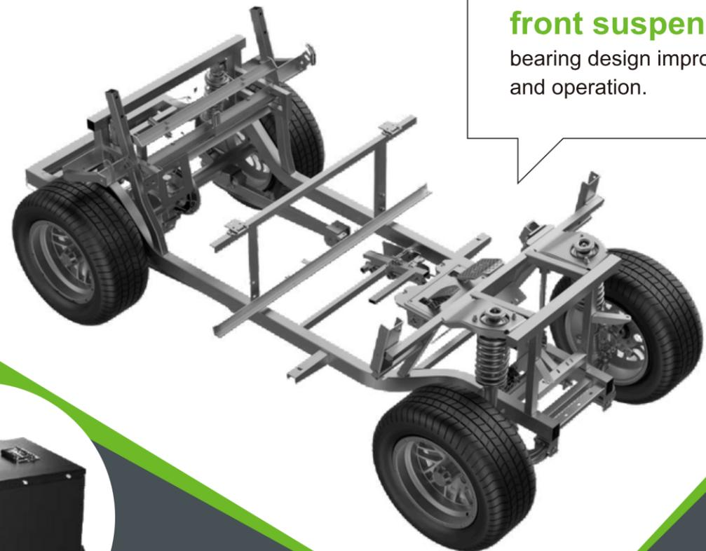
**McPherson independent front suspension** and non-load bearing design improve the ride comfort and operation.
